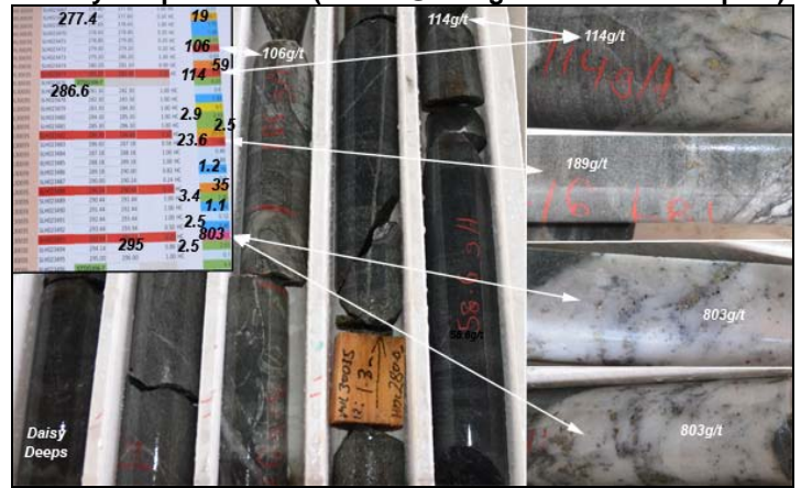
b. Daisy Deeps Drillhole (17.6m @ 23.6g/t: true width & topcut)
